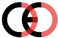
False CE Mark (too close)
