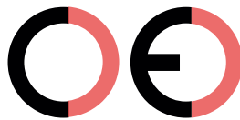
False CE Mark (too far)
