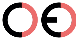
False CE Mark (too far)
