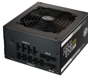
Fully modular cabling
