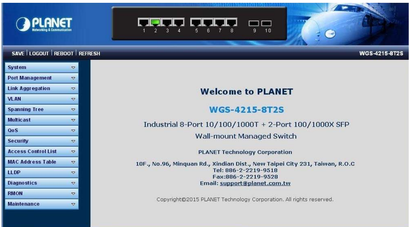
Figure 3-1-4 Web Main Screen of Managed Switch
