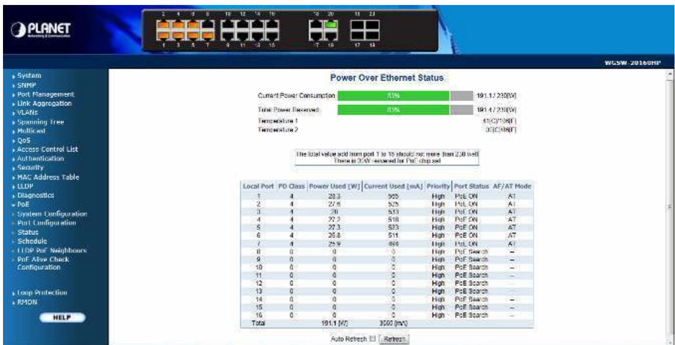
Figure 4-16-1: Power over Ethernet Status
