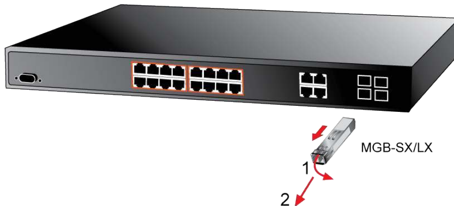
Figure 2-8: How to Pull Out the SFP Transceiver
