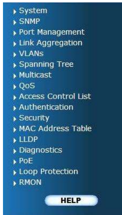
Figure 4-1-5: Managed Switch Main Functions Menu
