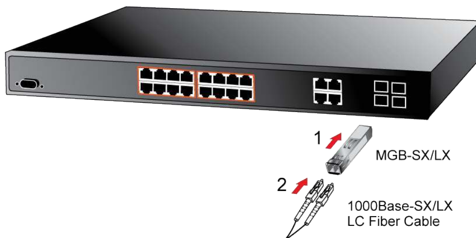
Figure 2-7: Plug-in the SFP Transceiver
