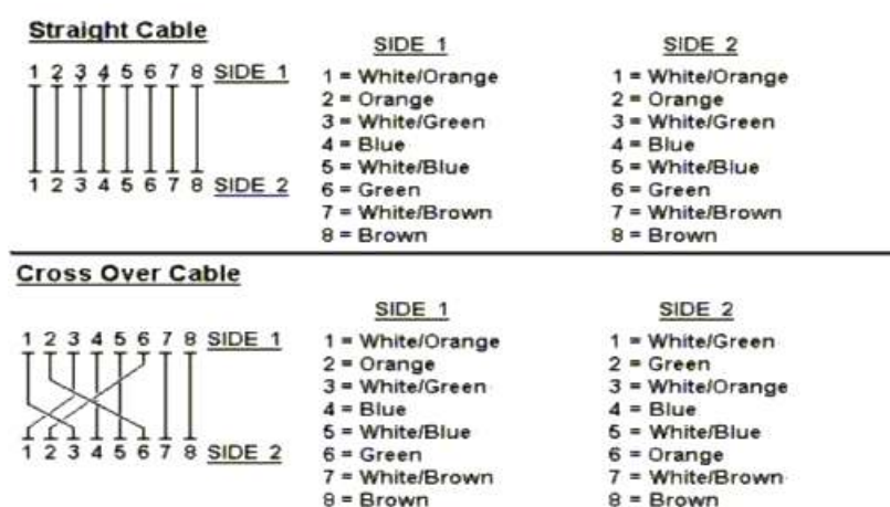
Figure A-1: Straight-Through and Crossover Cable
